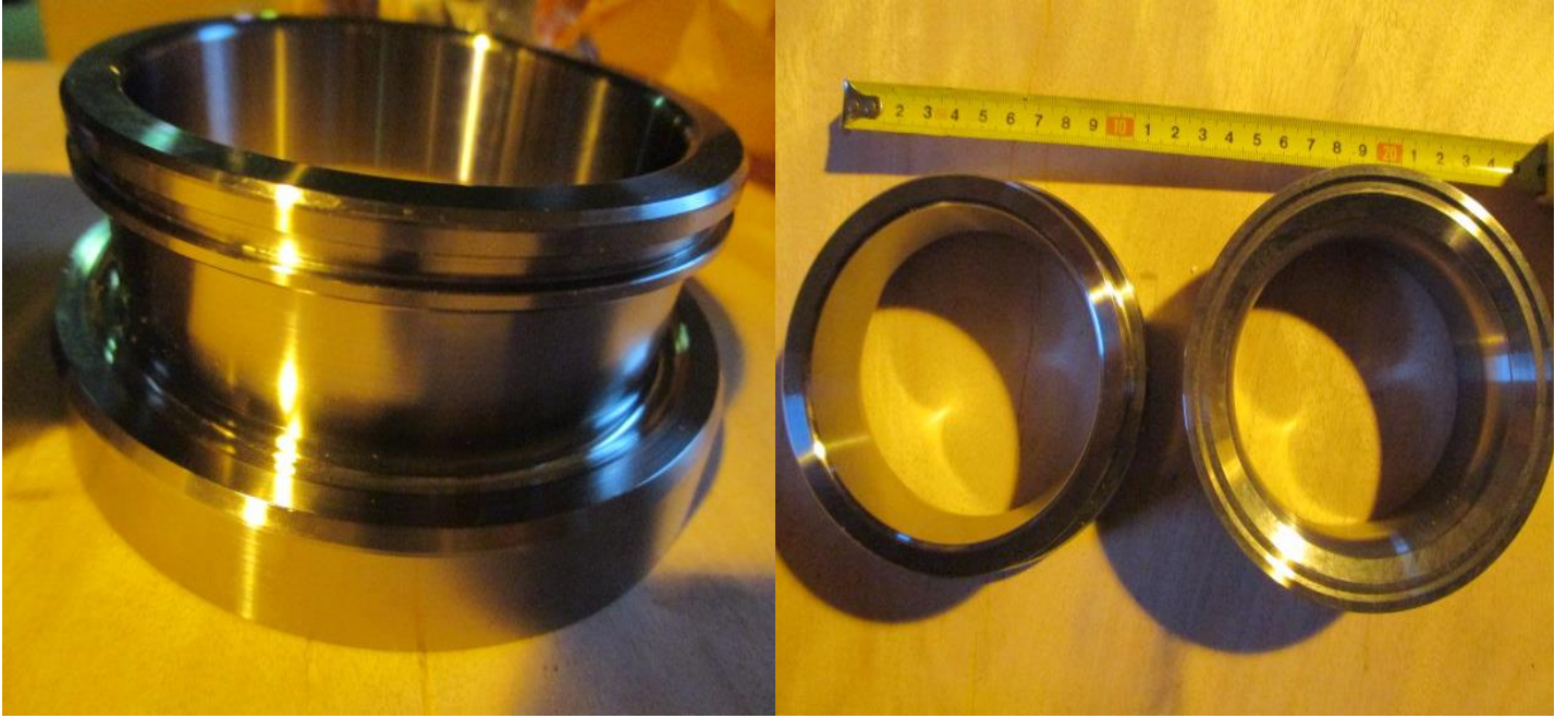
Valve seat (standard size) Maximum diameter - 121 mm Sealing ring seat place - 109 mm
